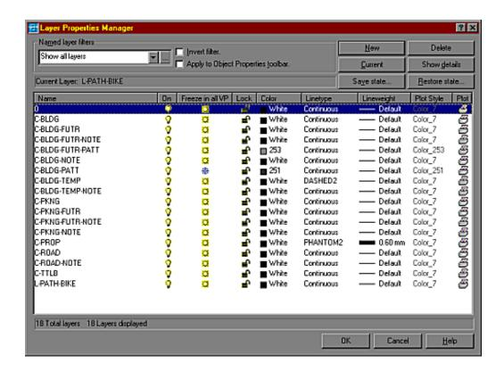
One advantage of establishing the CAD standard around a uniform layer dictionary is that it can be extended as needed using the same drafting conventions. The goal for master plan map maintenance over time is consistency in organization across map files, which enables graphic conformity and data reliability.
