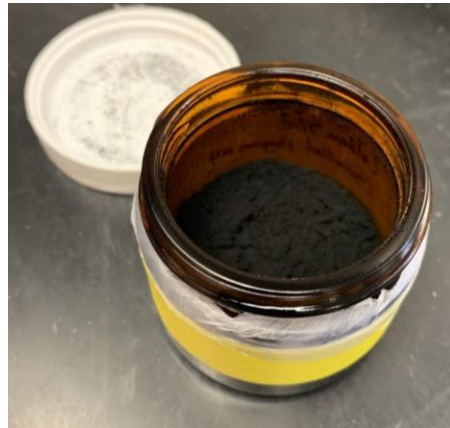
Pristine, cryomilled tire tread particles 32.2 \text{ um} \pm 25.5 \text{ um}
